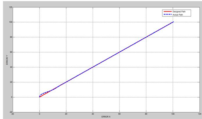
**Figure 10.** Straight line trajectory tracking control of the tractor
