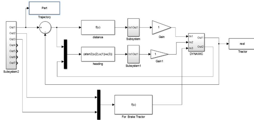
**Figure 9.** Simulation of dynamic model and controller via MATLAB/ Simulink Program
